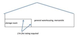
In this scenario, the exterior walls must be non-combustible or provide a minimum of a one-hour fire rating. A two-hour fire separation is required between the general warehouse/mercantile area and the chemical storage area. The ceiling of the storage room would require a two hours fire rating (both sides).
