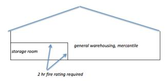
In this scenario, the exterior walls must be non-combustible or provide a minimum of a one-hour fire rating. A two-hour fire separation is required between the general warehouse/mercantile area and the chemical storage area. The ceiling of the storage room would require a two hours fire rating (both sides).
